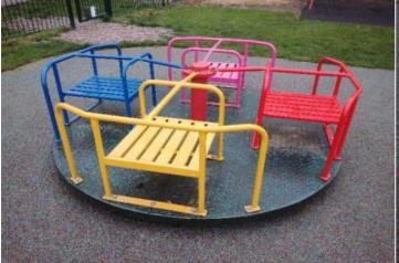
**Finding:** There is/are finger entrapment/s in the seats and the item fails to meet the requirements of BS EN 1176 Part 1 4.2.7.6 Entrapment of fingers
