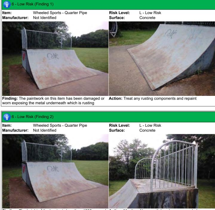
**Finding:** The height of the barrier is less than 1200mm and **Action:** Monitor - No remedial work recommended fails the requirements of BS EN 14974
