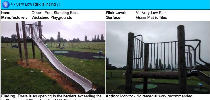
**Finding:** There is an opening in the barriers exceeding the **Action:** Monitor - No remedial work recommended width allowed (500mm) in BS EN 1176, and no guardrail has been provided; this is a low risk failure and no remedial action is required
