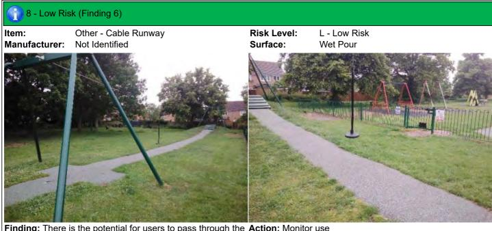
Finding: There is the potential for users to pass through the Action: Monitor use freespace of the cableway when entering or exiting the play area
