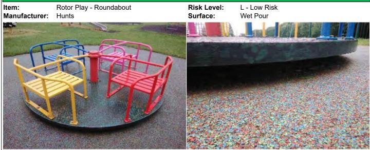
**Finding:** The underside of the rotating platform shall be smooth for the first 500mm towards the axis to comply with the requirements of BS EN 1176 Part 5
