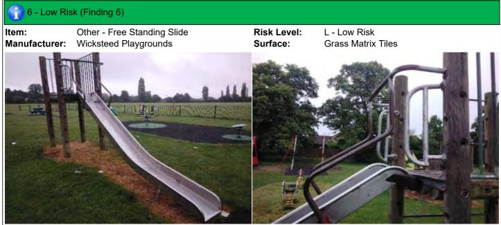
Finding: The paintwork on this item has been damaged or Action: Treat any rusting components and repaint worn exposing the metal underneath which is rusting
