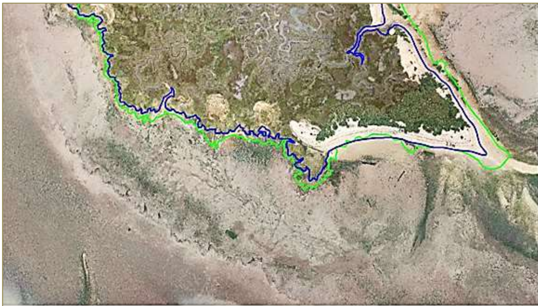
Figure 10. Edge erosion of saltmarsh, southern margin of Cobmarsh Island, between 2014 (green line) and 13 September 2021, two months before recharge delivery, (blue line). The width of loss during this seven-year period generally ranged between 3m and 5m (0.43m – 0.71m annual rate of loss), with a maximum edge loss of 11m (1.58 annually).
