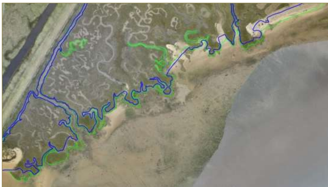
Figure 12. Edge erosion of saltmarsh, south-eastern margin of Old Hall between 2014 (green line) and 13 September 2021, two months before recharge delivery began (blue line). The width of loss during this seven year period generally ranged between 2m and 3m (0.28m – 0.43m annually), with a maximum loss of 9m in places (1.28m annually).
