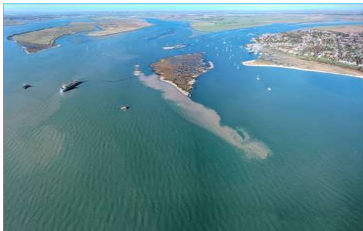
Figure 5. Cobmarsh Island: sediment plume deriving from pipeline delivery 1 from the trailing suction hopper dredger, Sospan Dau.
