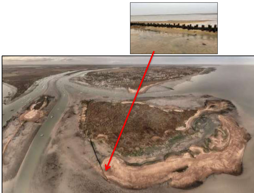
Figure 29. View NE with Packing Marsh Island to the west and Mersea Island in the background. The Mersea Fleet cuts between the two islands. The fence runs from north to south across the western foreshore. The photo was taken on 16 January 2023, just over one year after recharge was completed, on 27 December 2021. Inset shows the movement of material around the southern end of the fence on 12 January 2023 (looking west).
