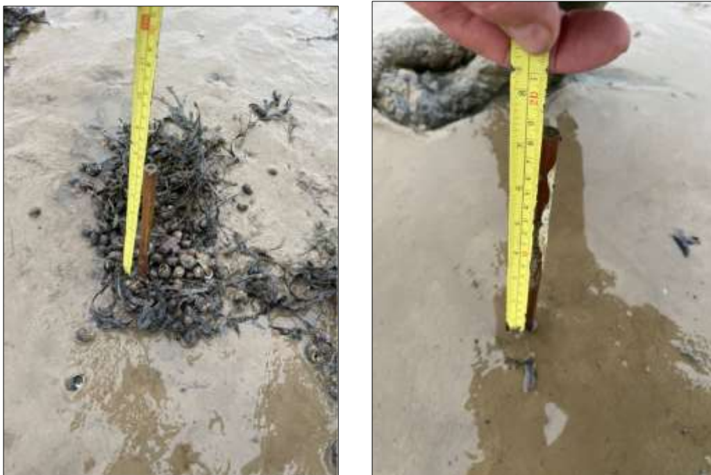
Figure 23. Taking siltation readings. At Old Hall (left), brown seaweed had wrapped around the cane and had to be moved to obtain the reading. Live common periwinkle (edible periwinkle: Littorina littorea ) were clustered beneath the seaweed. A reading of 184mm was taken at the location on the right (Cobmarsh Island) giving an accretion measure of 16mm.
